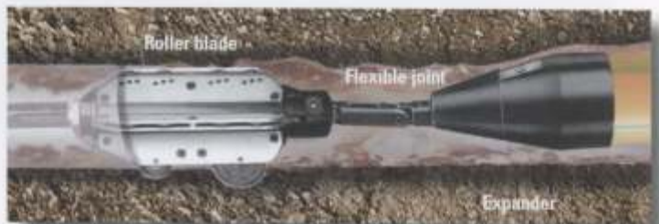
The roller blade cuts pipes made of tough materials (plastic, steel, cast iron).
