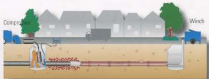
Grundocrack is driven by compressed air. A winch pulls and supports the bursting process
