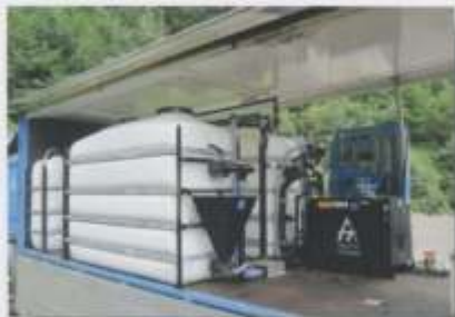
Bentonite mixing system MA 010 for all HDD rigs
